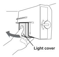
2. Remove the 2 screw, and pull the Lamp out.
