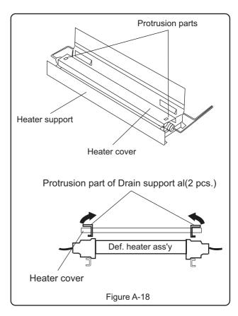
3. Open Def.heater fixed part of Heater support al to the right and left, then remove Def.heater ass'y.
