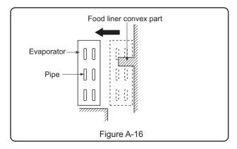
4. Pull the Evaporator for remove as shown in Figure A-16.
