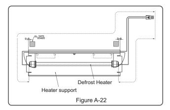
8. Roll the leading wire Sealer to Lead wire Defrost Heater.
