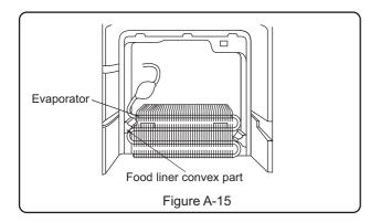
As shown in Figure A-15, pull the upper part of Evaporator toward you, pull it diagonally so that the pipe of Evaporator does not contact the convex part of food liner.
